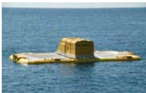
Figure 21: No.3 prototype system of wave power generation system using gyro moment (45 kW) 26
